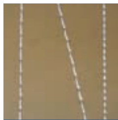
Stitch sample. Max. stitch length: 8.0 mm (3.2 SPI)
